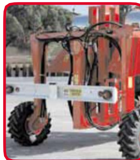
Carreggiata posteriore variabile Variable rear track gauge
